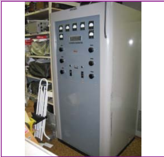
PHOTO 1: Gates BC-250GY 250-watt AM Broadcast Transmitter donated to NEHRS by Frank Gentges, KOBRA.
